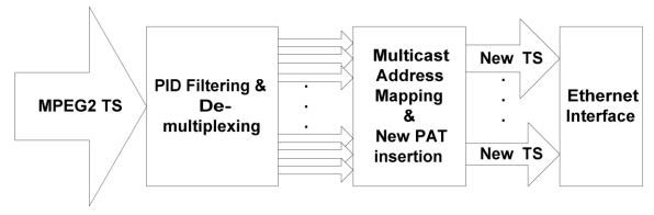
Figure 1 – Novra Receiver Enhanced Capability
