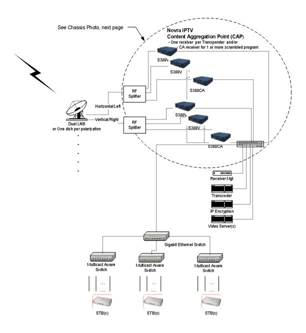
Figure 2 - IPTV Network Diagram Example
